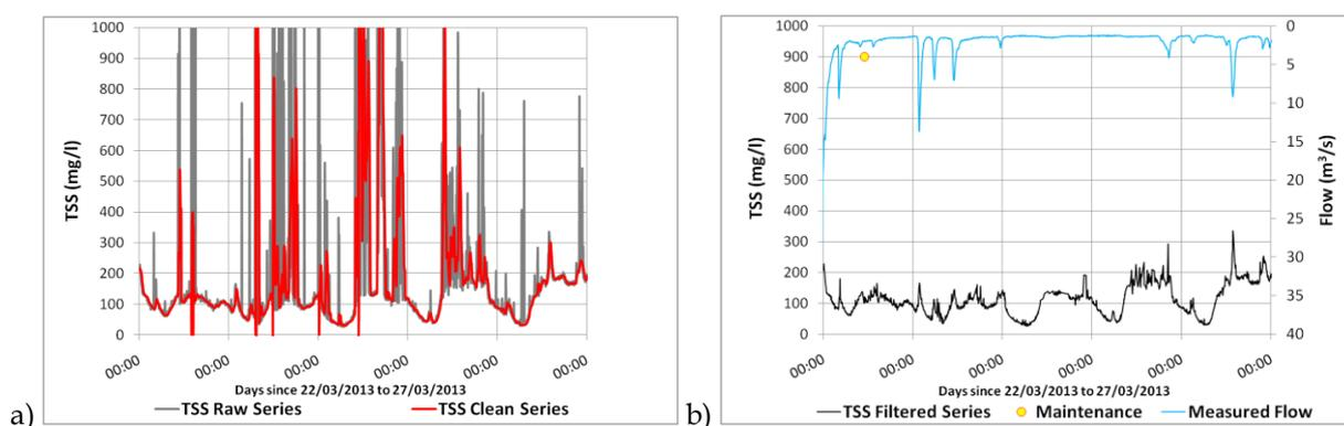
Figure 2 – TSS monitoring during a rainy period and comparison between a) data provided by the S::CAN spectrophotometric probe and b) data stored after processing and treatment.
