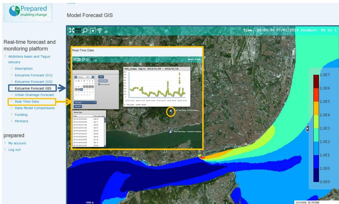
Figure 3 – Global view of interface, showing faecal concentration forecasts and the location of the PREPARED network stations
